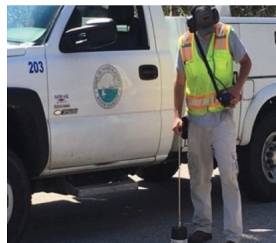
Figure 4: Leak Detection Listening Stick
