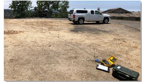
Figure 1: In-Situ Soil Resistivity Testing Setup
