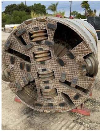
Microtunneling Boring Machine - Cutting Head
