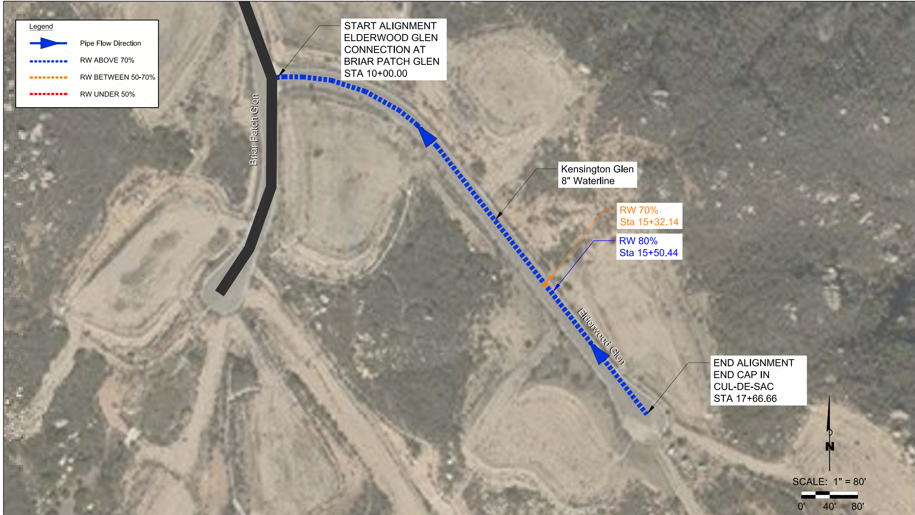
FIGURE 2: KENSINGTON GLEN DEFECT LOCATIONS
