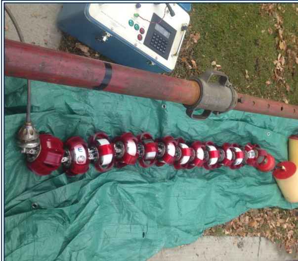
Figure 2a: PICA's SeeSnake tool used for smaller diameter inspections.
